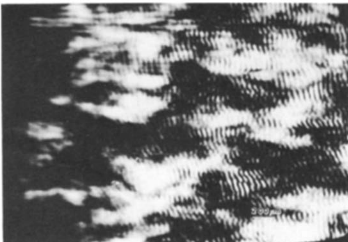
Figure 15 Micrograph of a well bonded strip delaminated to two layers. The large white bonded areas indicate by their size that bonding is associated with areas of high silicon concentration.
